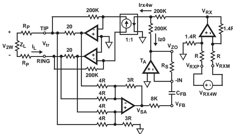
FIGURE 12. SCHEMATIC FOR 4-WIRE TO 2-WIRE GAIN DERIVATION
