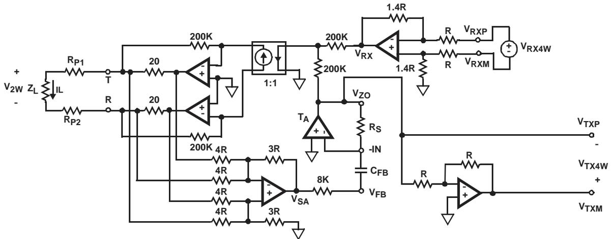
FIGURE 14. SCHEMATIC FOR 4-WIRE TO 4-WIRE GAIN DERIVATION
