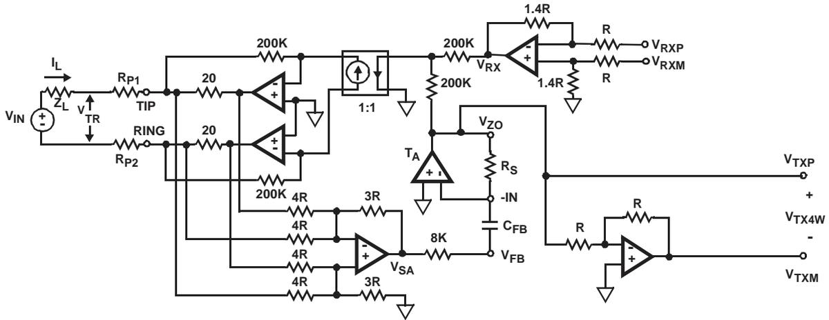
FIGURE 13. SCHEMATIC FOR 2-WIRE TO 4-WIRE GAIN DERIVATION
