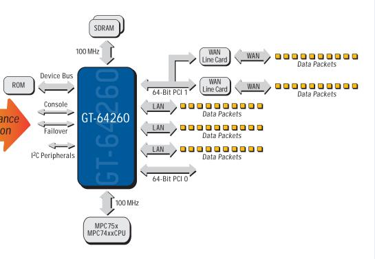
standards and integrate MAC functionality with a dual speed MII/RMII interface. The GT-64260 supports Auto-Negotiation of port speed (10 or 100 Mbps) and communications mode (half or full-duplex) through the PHY. Up to 8K MAC addresses can be up filtered with on-chip logic allowing a packet to be discarded at the MAC level before precious bandwidth is wasted on storing and analyzing the packet by the CPU.
