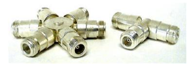
Microlab/FXR DA through DF series power dividers are miniaturized multi-terminal devices designed to separate or combine RF signals. They employ resistive elements to match one or more terminals to 50 ohms. Careful design of resistive elements and impedance matching techniques permit the use of these dividers at frequencies to 1.5 GHz and higher.
