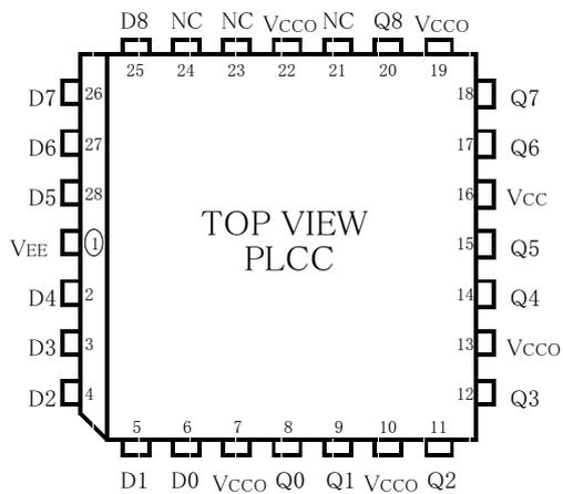
\*All VCC and VCC0 pins are tied together on the die.
