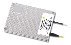
The JDS Uniphase 54TR series transponder integrates optics and electronics in an OC-48 (2.5 Gb/s) time division multiplexing (TDM) transponder module. Multisource agreement (MSA) compatible and designed for operation at 1310 and 1550 nm, it can be used across a variety of optical fiber systems.
