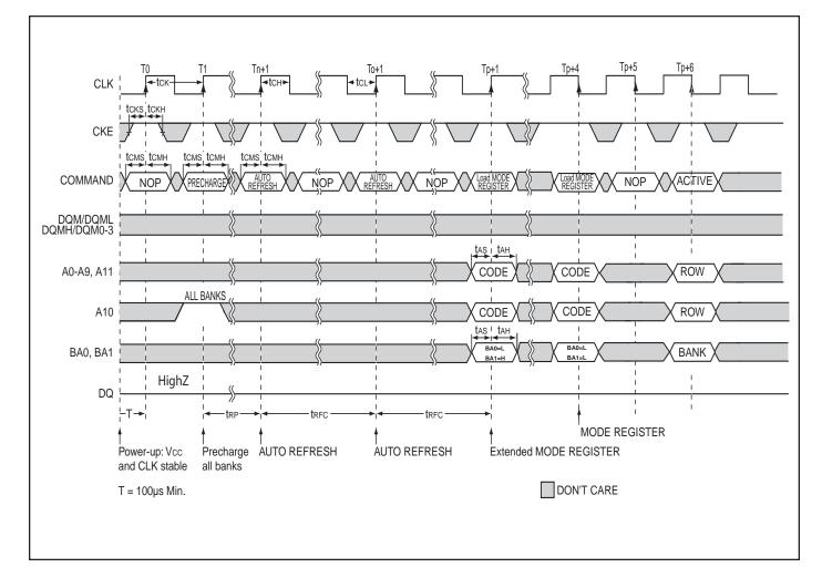
**Note:** The Load Mode Register for both Mode Register / Extended Mode Register and two Auto Refresh Commands can be in any order. However, all must occur prior to an Active Command.
