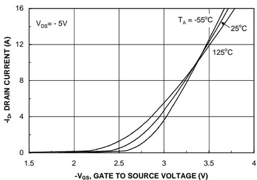
Figure 5. Transfer Characteristics.
