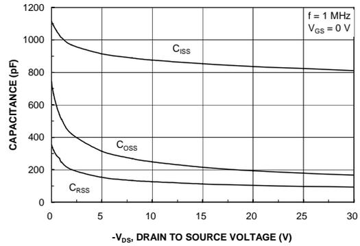
Figure 8. Capacitance Characteristics.
