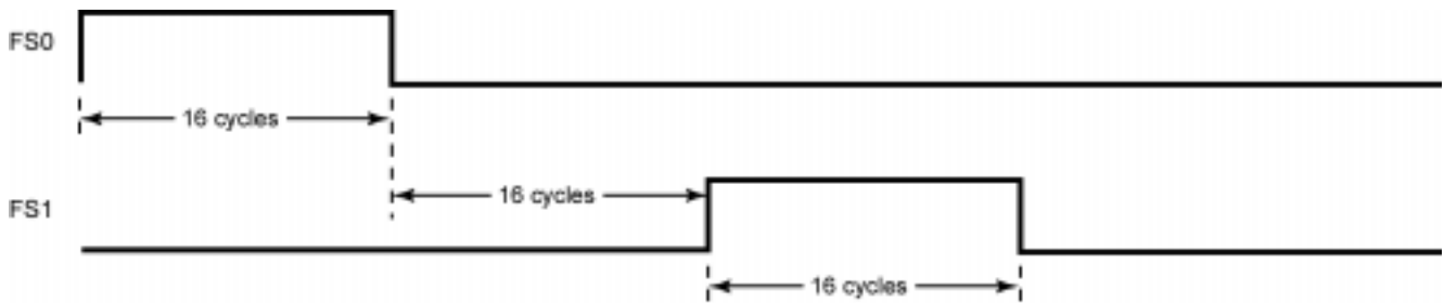
Figure 21. 16-Bit CODEC Frame Synchronization
