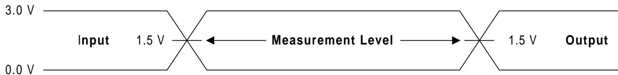
Figure 14. Input Waveforms and Measurement Levels
