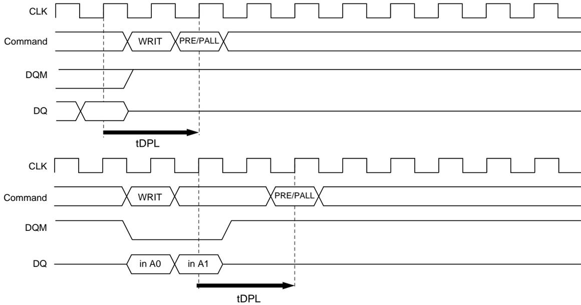
**WRITE to PRECHARGE Command Interval (same bank) (BL = 4 (To stop write operation))**
