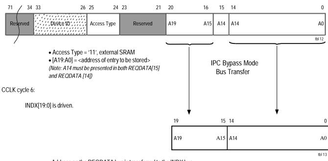
• Address on the REQDATA bus is transferred to the INDX bus. REQDATA[20:16],[14:0] | INDX[19:15],[14:0]
