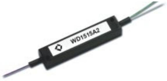
The WD1515 A2/D2 add/drop filter couplers are designed for Dense WDM network drop-and-insert applications. The minimum channel spacing is 200 GHz and the channels are centered on the 100 GHz ITU wavelength grid. As many as 50 ITU wavelengths within the erbium doped fiber amplifier gain band are available.
