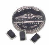
The Model SM500 is an ultra-broadband, surface-mount DC Block designed for use in 20 Gb/s systems. It passes very fast risetime pulses with a minimum of waveform distortion. The risetime is only 10 ps, and the -3 dB bandwidth extends over many decades from 7 kHz to 35 GHz. The small size and low cost enable system design-
