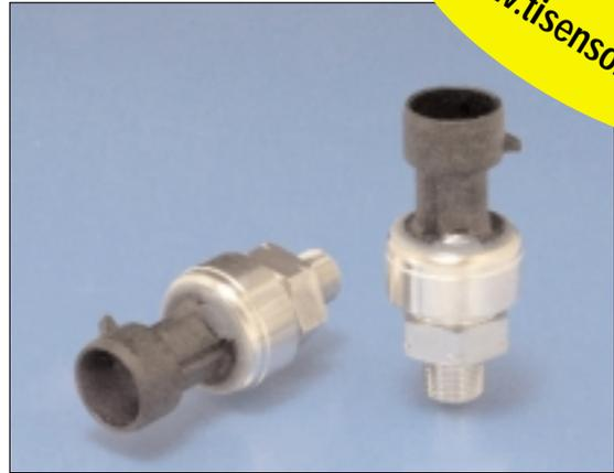
The 61CP Series transducer is ideally suited for environmentally demanding OEM industrial applications. This is a high accuracy, 0-5 Vdc high-level output design that requires no end user amplification. Output is ratiometric to supply
