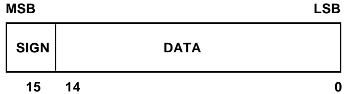
Figure 31a. Single 6Precision Fixed-Point Data
