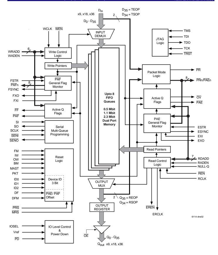
Figure 1. Multi-Queue Block Diagram
