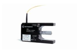
JDS Uniphase manual backreflectors provide precise levels of return loss to transmitters, which allows measurements of system sensitivity or system degradation as a function of backreflection. When used with a transmitter/receiver pair and characterization equipment, the backreflectors can be used to establish the magnitude of reflections that significantly degrade transmission system performance and to characterize the problems they cause.
