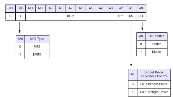
\* All bits in RFU address fields must be programmed to Zero, all other states are reserved for future usage \*\* This part do not support /QFC function, A2 must be programmed to Zero.
