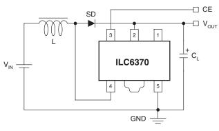
L:  $100\mu$ H SD: Schottky diode C<sub>L</sub>: 47µF 16V (Ceramic or Tantalum Capacitor)
