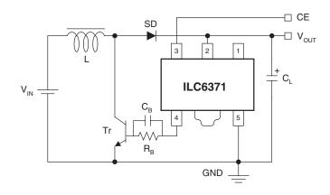
L: 100 $\mu$ H SD: Schottky diode C<sub>L</sub>: 47 $\mu$ F 16V (Ceramic or Tantalum Capacitor) R<sub>B</sub>: 1k $\Omega$ C<sub>B</sub>: 3300pF Tr: 2SC3279, 2SDI628G
