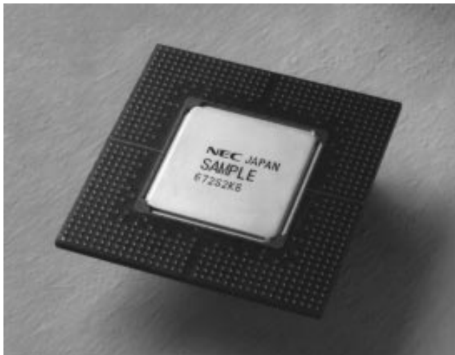
Figure 1. BGA Package Examples
