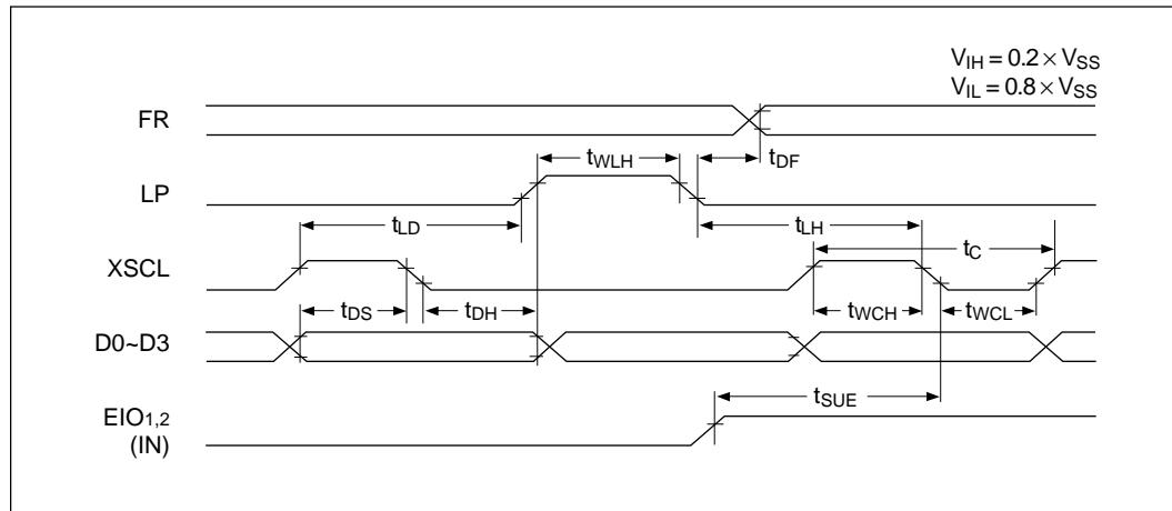
$V_{ss} = -5.0V \pm 0.5V$ ,  $T_a = -40$  to  $85^{\circ}\text{C}$
