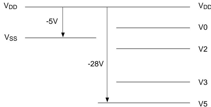
Note 4. When logic power becomes floating state or if V<sub>SS</sub> = -2.6 or beyond while the LCD driver power source is being applied, the LSI may be permanently damaged and avoid such circumstances.
