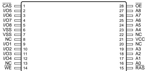
28 Lead TSOP-I PIN CONFIGURATION Top View
