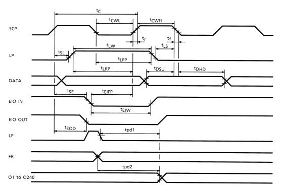
TEST CONDITIONS (1) ( $V_{SS} = 0 \text{ V}, V_{DD} = 4.5 \text{ to } 5.5 \text{ V}, V_{CC} = 14 \text{ to } 42 \text{ V}, Ta = -20 \text{ to } 75^{\circ}\text{C}$ )
