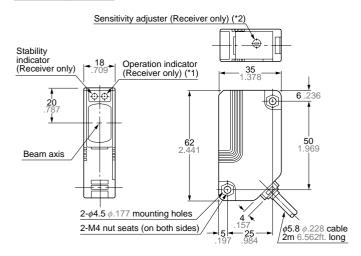
(\*1): It is substituted with the power indicator on the emitter of UZE100□.
