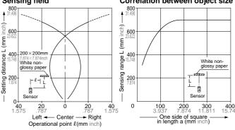
As an object size becomes smaller than the standard (White non-glossy paper 200  $\times$  200mm  $7.874 \times 7.874$ inch), the sensing range shortens. The left graph is plotted on condition with the sensitivity having been adjusted at 700mm 27.559inch of the sensing distance exactly detectable with the white non-glossy paper of 200 × 200mm 7.874 × 7.874inch.
