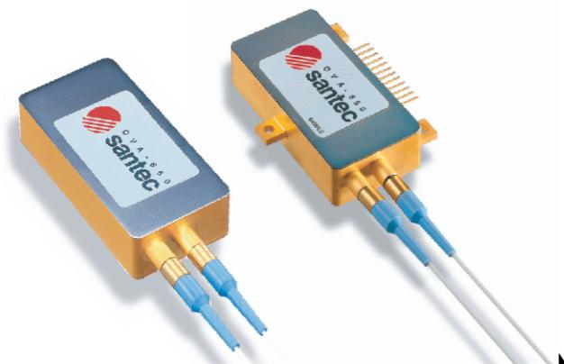
The OVA-650 is a compact variable optical attenuator that uses a stepper motor for accurate electrical control. The unit has high resolution, low insertion loss, low PDL, and exhibits extremely low wavelength dependence. Two package designs are available with effective height of 12mm and 8mm (Dual-line pins on the bottom, Single-line pins on the side with screw tabs) respectively. This device can be easily mounted onto a printed circuit board for system integration.
