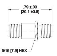
Note: Dimensions in Brackets are Expressed in Millimeters and are for Reference Only. Gold plated connectors are also available.
