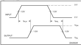
Waveform 1. Waveforms Showing the Input (An) to Output (Yn)
