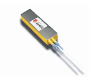
The OTF-655 is a compact, tunable filter module that incorporates a stepper motor for accurate wavelength selection. The device utilizes Santec's unique polarisation independent, linear sliding technology to achieve accurate wavelength tuning whilst maintaining constant optical properties over the entire wavelength range. The device is hermetically sealed with an effective height of only 7.1mm. It is suitable for PCB mounting and system integration.
